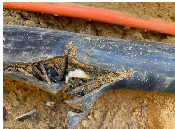
Damaged section of LV mains cable which had been impacted by another star picket causing the power outage.
